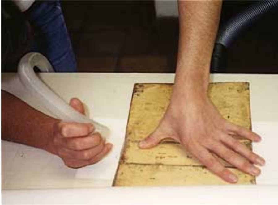
Illus. 8 Yapp edges being formed with the vacuum table
